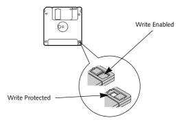
Figure 4-3 Floppy Disk Write Protect
